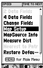
'Map Setup' allows you to change map orientation, background map detail, on-screen Jeppesen data, text size, etc.
